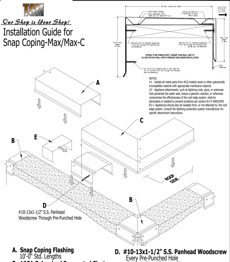
**B. 16GA Galvanized Segmented Cleat** 12" Width, Spaced 40"o.c. MAX.
