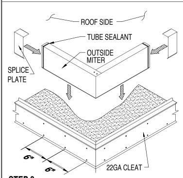
STEP 2 : Installing Fascia Cover LT Miters
