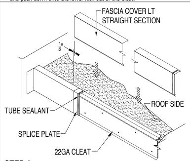
STEP 4: Installing Fascia Cover LT Straight Lengths
