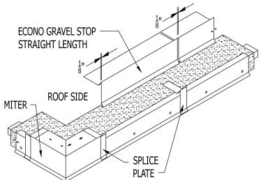
**STEP 4**: Installing Econo Gravel Stop Straight Lengths
