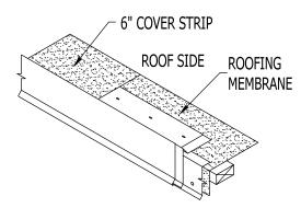
**STEP 5: Installing Approved Roofng Membrane**Install 6" Cover Strip per roofing manufacturer's instructions.
